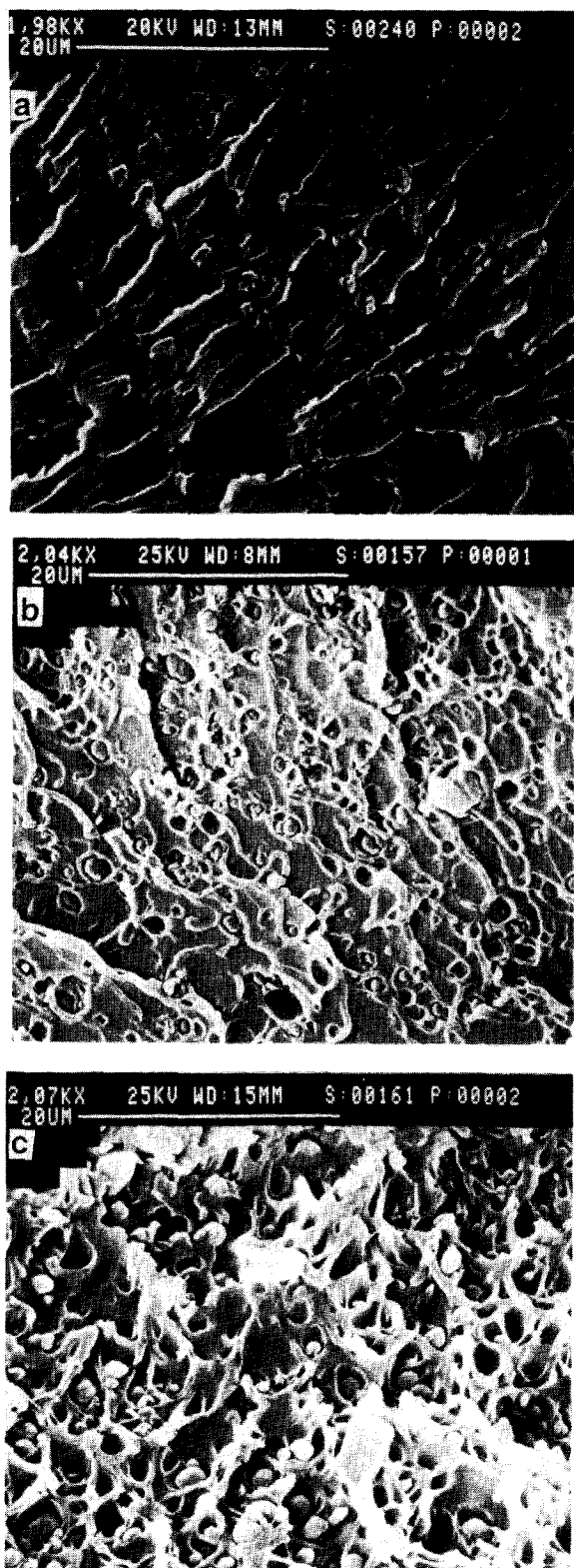
Figure 8 S.e.m. micrographs of the fractured surfaces of extruded Ultem/Granlar films of various blend compositions: (a) Ultem/Granlar 90/10; (b) 80/20; (c) 70/30
