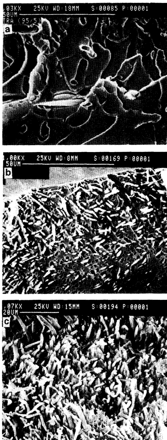
Figure 7 S.e.m. micrographs of the fractured surfaces of extruded Ultem/Vectra films of various blend compositions: (a) Ultem/Vectra 95/5; (b) 90/10; (c) 70/30
